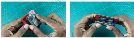
Fig. 5.7: ESP32 board to the adapter connection
