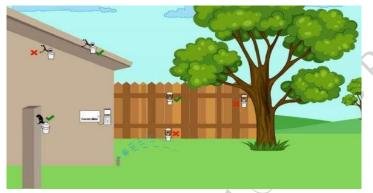
Fig. 1.3: Suitable location for outdoor sensors
