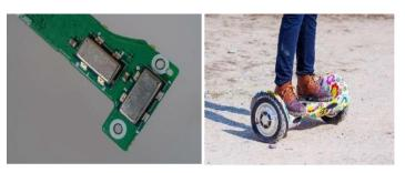
Fig. 3.11: Use of Gyroscopic sensors
