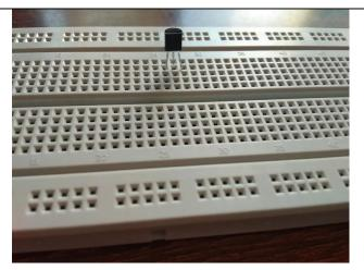
Fig.3.25: transistor on breadboard
