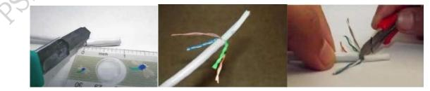
(a) Stripping the cable (b) Pull wires backward (c) Cut the core Fig. 2.9: Preparation of the Cable
