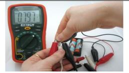
Fig.3.22: TMP36 sensor testing at high temperature
