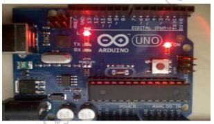
Fig.2.6: Tx and Rx LEDs on Arduino board
