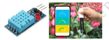
Fig. 3.12: Humidity sensor and Humidity sensor device
