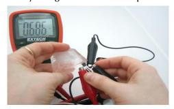
**Fig.3.23: TMP36 sensor testing at low temperature** As an ice-cube is pressed against the sensor, temperature drops down to 18.6°C / 65.5°F.
