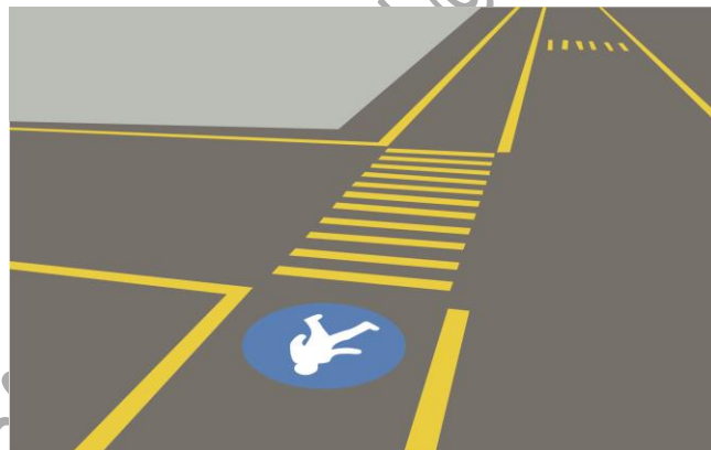
Fig.: 5.3 Yellow Demarcation for Pedestrian Pathway
