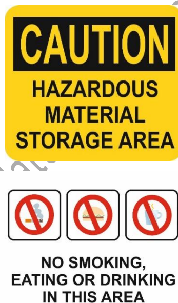
Fig.: 2.18 Safety signs at storage area of flammable material and chemicals
