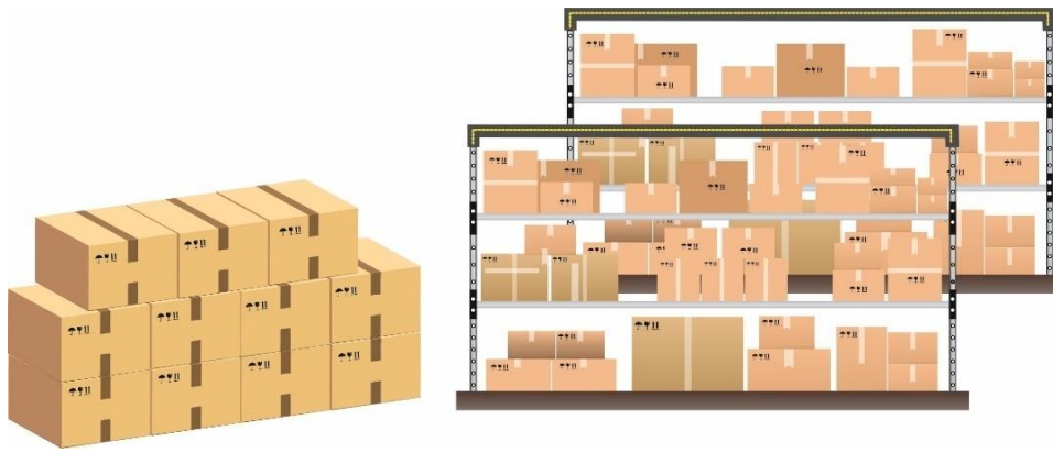
Fig.: 2.9 Block Stacking
