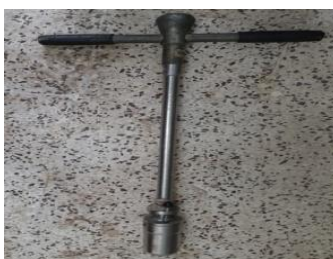
Figure 2.5: Sampler with core
