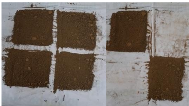
Figure 2.9: Quarter method of soil sample preparation
