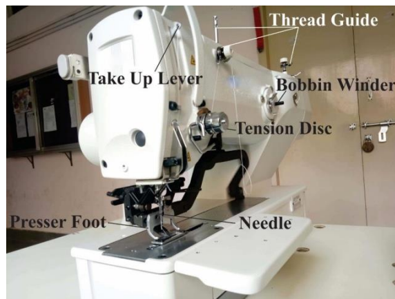
Fig 5.3: Parts of button sewing machine
