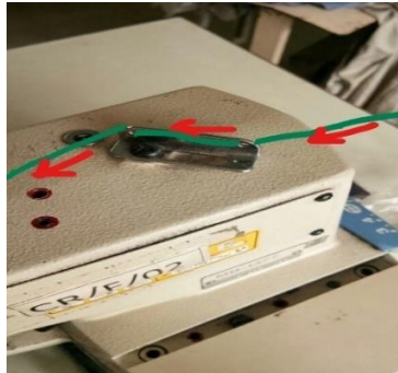
Fig.5.7: Button sewing machine threading- step2
