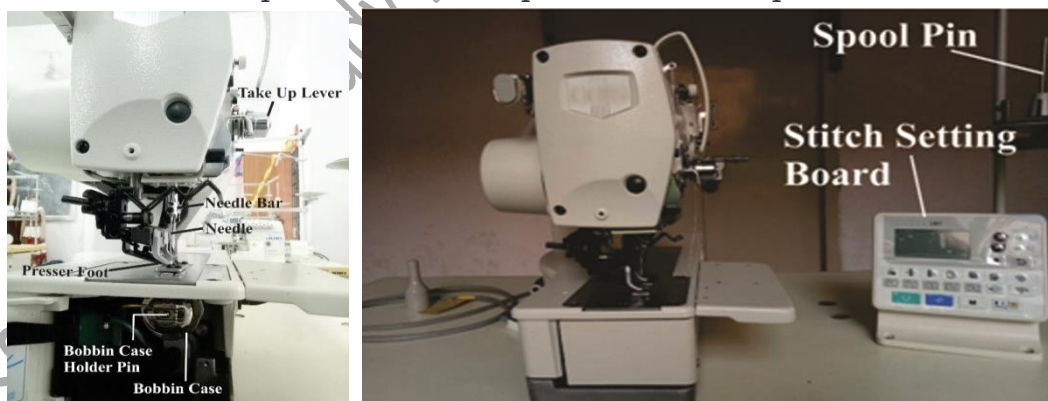
Fig 5.4 (a) (b): Button sewing machine and its parts
