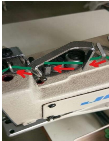
Fig.5.11: Button sewing Machine threading- step6
