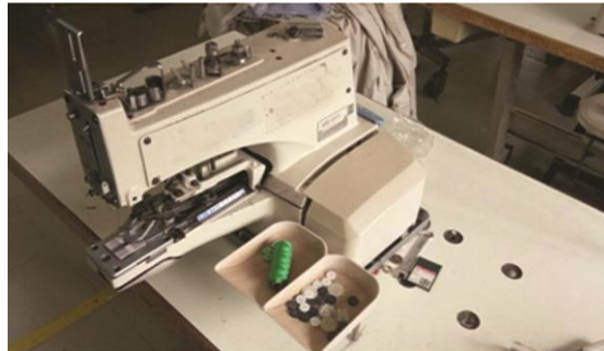
Fig 5.5: Button Sewing machine preparation
