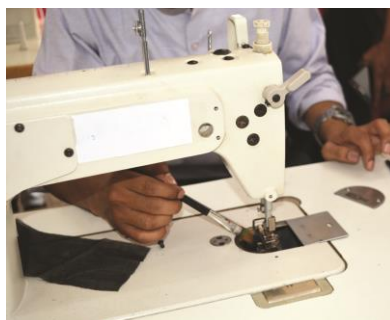
Fig. 6.4: Cleaning of bobbin case
