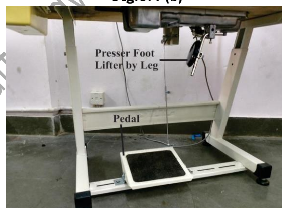
Fig.3.4 (a, b, c): Details of the SNLS machine
