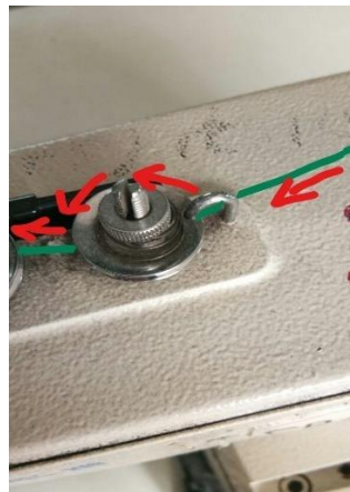
Fig.5.8: Button sewing machine threading- step3
