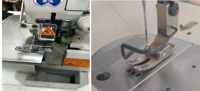
Fig.3.10 (a), (b): Various needle guards
