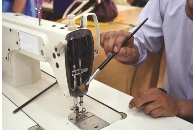
Fig. 6.5: Cleaning of face plate area
