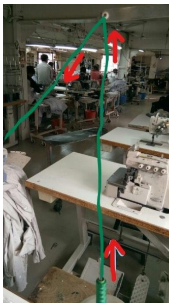
Fig.5.6: Button sewing machine threading-step1
