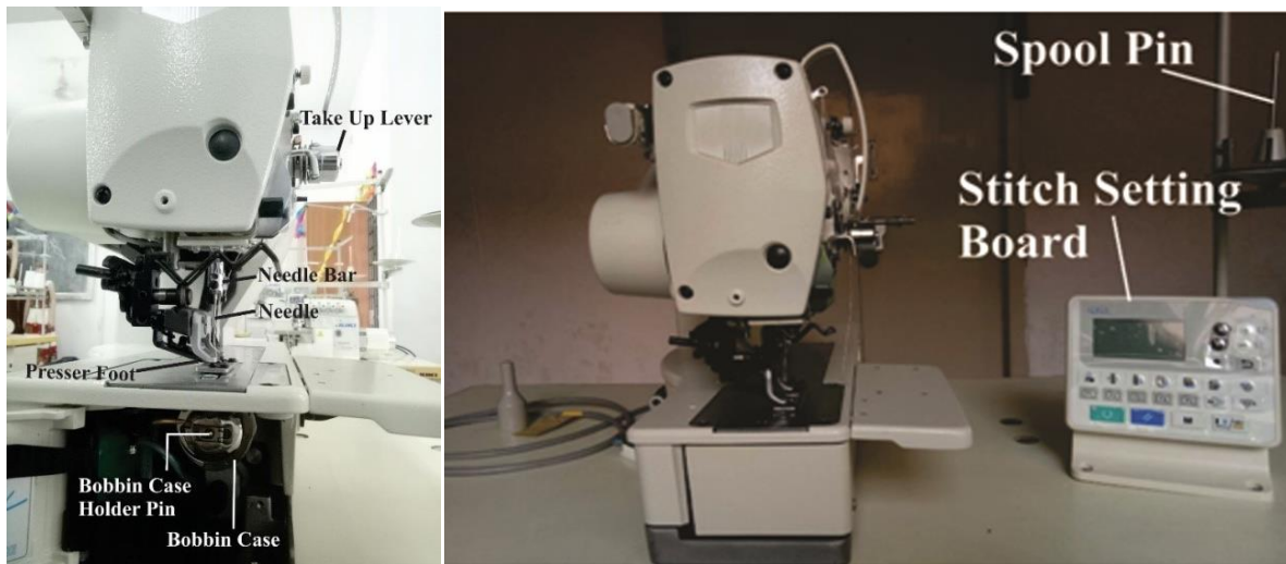
Fig.5.21 and 5.22: Parts of buttonhole sewing machine
