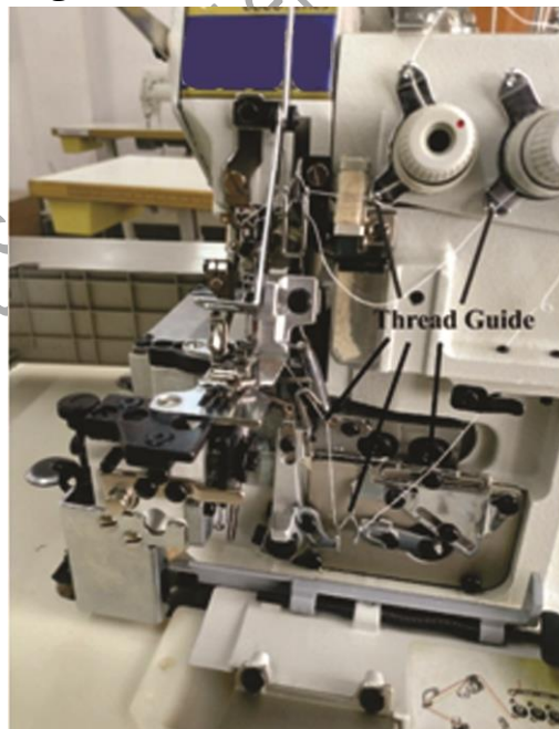
Fig.3.13: Steps of threading the over lock machine
