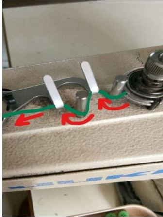
Fig. 5.10: Button sewing machine threading- step5
