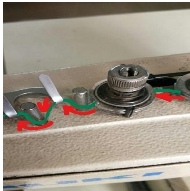
Fig.5.9: Button sewing machine threading- step4
