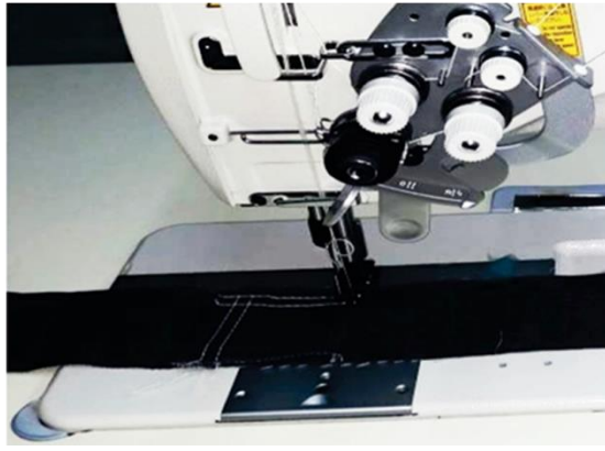
Fig.3.2: Double needle lock stitch machine
