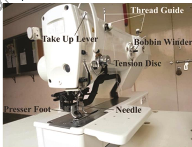
Fig. 5.20: Parts of buttonhole sewing machine
