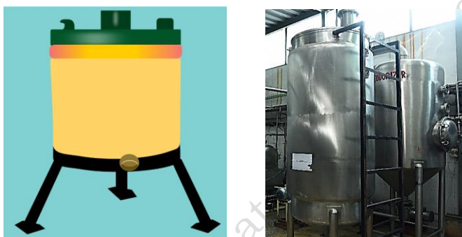
Fig. 2.9: Blancher for Small Scale and Industrial Scale Soybean Processing Unit
