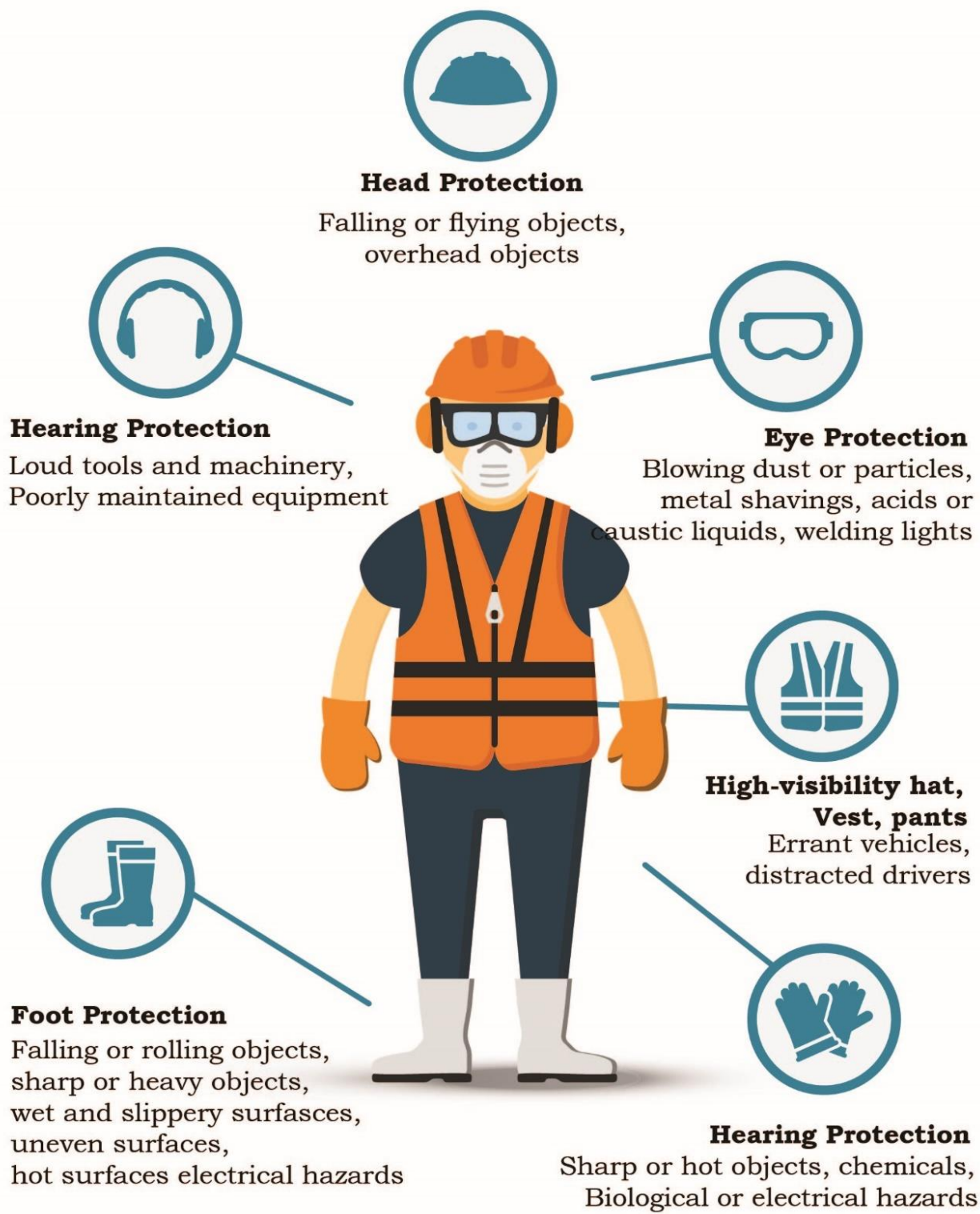
Fig. 3.23 Personal protective equipment (PPE) kit for workers
