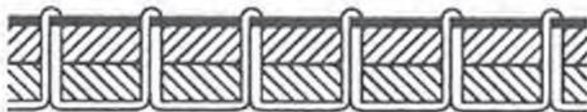
Fig. 2.54: Seams when the upper tension is too tight
