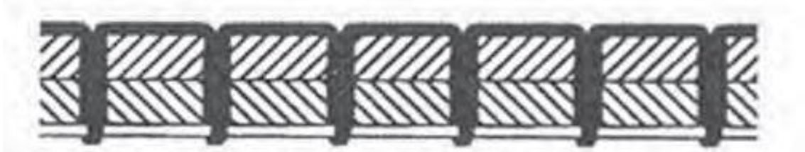
Fig. 2.53: Seams when the upper tension is too loose
