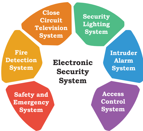
Fig. 3.5: Components of an electronic security system
