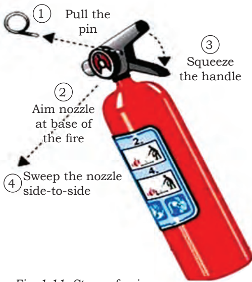
Fig. 1.11: Steps of using a fire extinguisher
