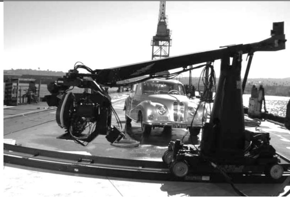
Fig. 1.2 Real-time Motion Control System on location with curved track
