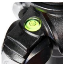
Fig.2.7 (b) Bubble level for tripod balancing
