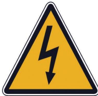
Fig. 5.6: Electricity hazard sign
