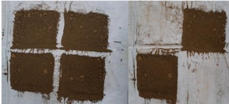
Fig. 4.7: Quarter method of soil sample preparation
