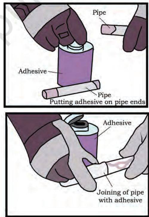
Fig. 4.27: Joining of elbow after application of solvent
