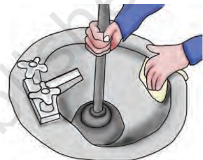
Fig. 6.12: Removing clogs in a washbasin
