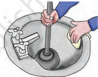
Fig. 5.12: Removing clogs in a washbasin
