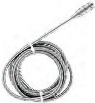
Fig. 5.13: Use of tools for removing clogs
