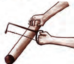
Fig.1.10: Cut and clean the edges of the pipe
