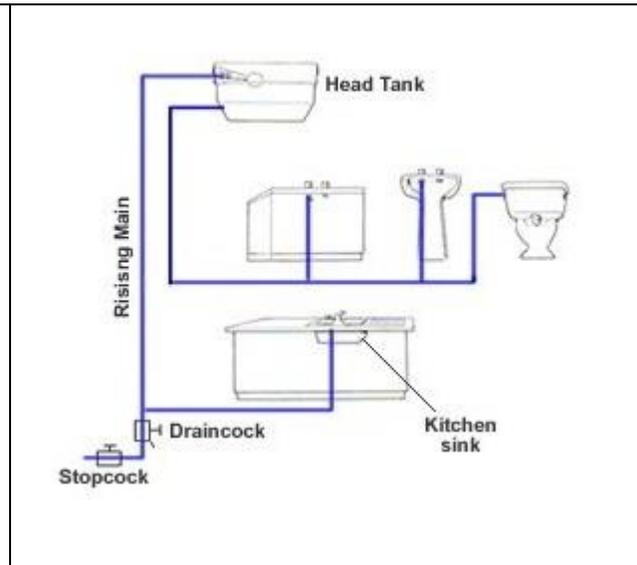
Fig 1.8 Indirect Water supply system
