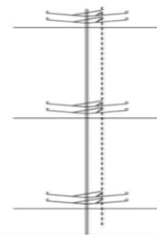
Fig 1.5 One-pipe system
