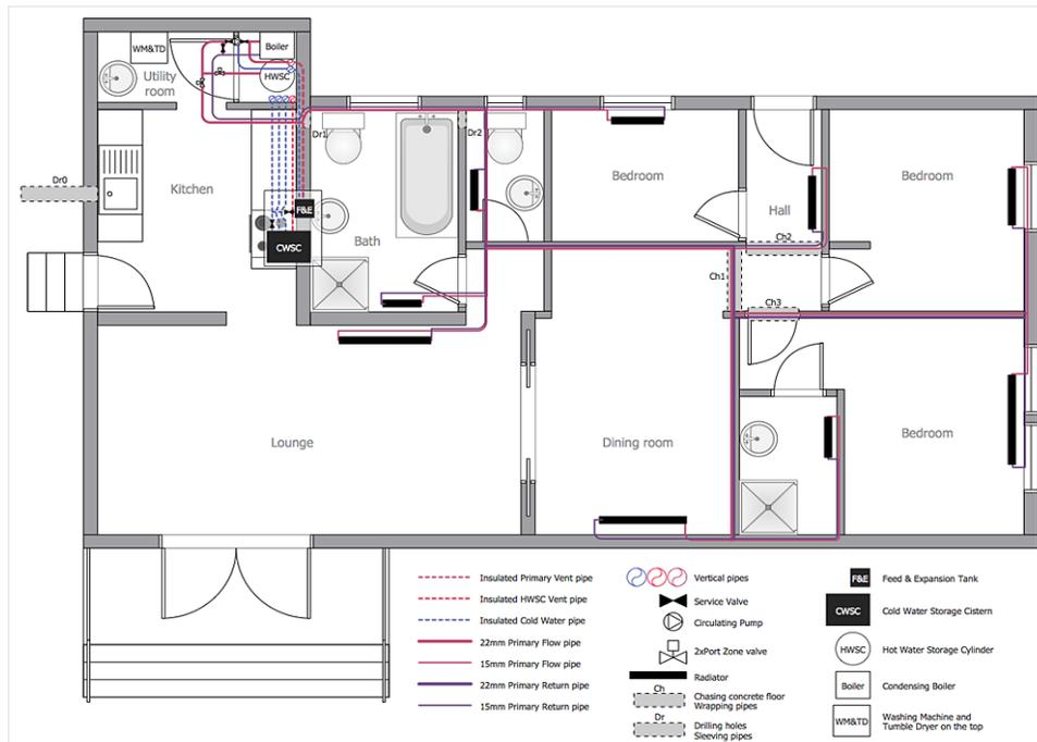
Fig 3.1 Plumbing Drawing of a residential house
