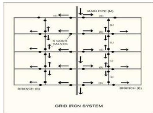
Fig 4.4 Grid Iron System
