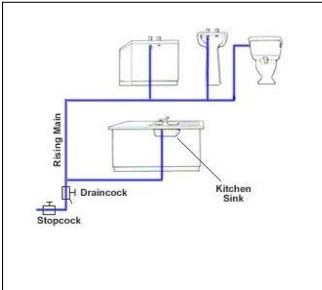
Fig 1.7 Direct Water supply system
