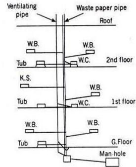
Fig 1.4 Partially vented Single stack system
