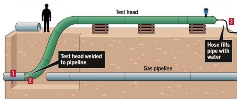
Fig 4.15 Pressure Test
