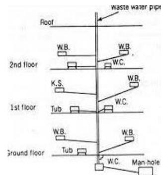
Fig 1.3 Single stack system
