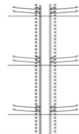
Fig 1.6 Two -pipe system
