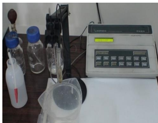
Fig. 2.6: 9A Ph Meter used to measure the acidity or basicity of a solution
