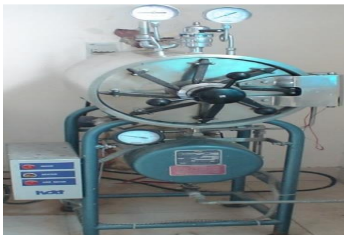
Fig. 2.5: An autoclave used to sterilize nutrient media, glassware, equipment, and other materials
