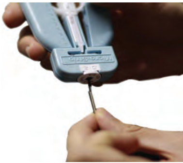
Fig. 4.17: Stripping of optical fibre cable
