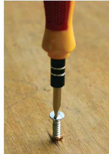
Fig. 4.2: Tip of the screwdriver is put into the screw head
