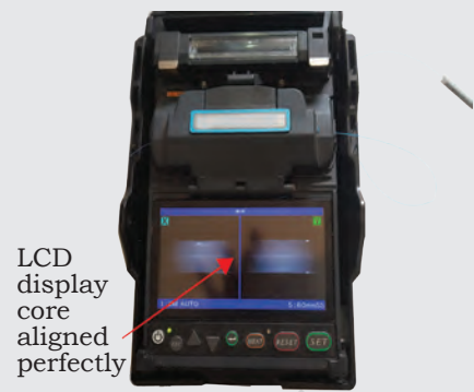
Fig. 5.34(c): Core aligned perfectly
