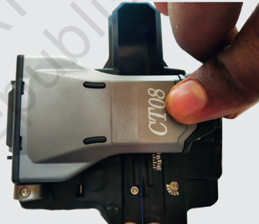
Fig. 5.23(b): Cleave it by pressing cap
