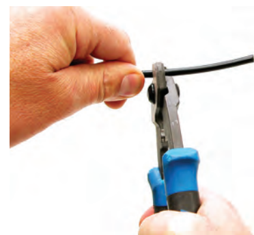
Fig. 4.15: Pulling out the jacket from cables
