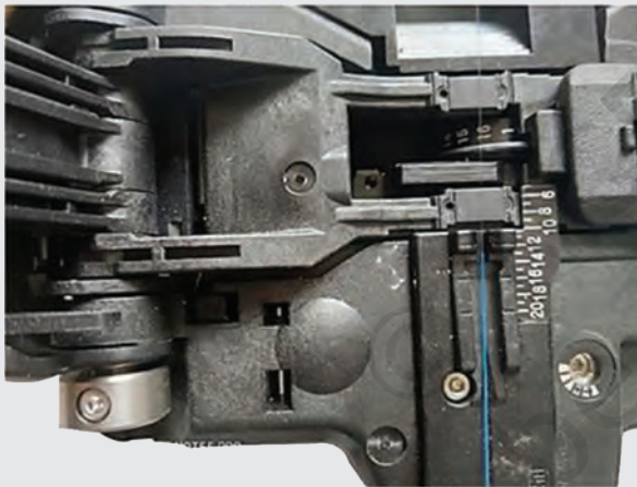
Fig. 5.23(a): Place the fibre in cleaver and adjust the blades
