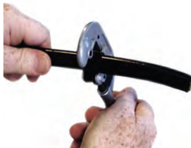
Fig. 4.14: Rotation of tube cutter around the cable
