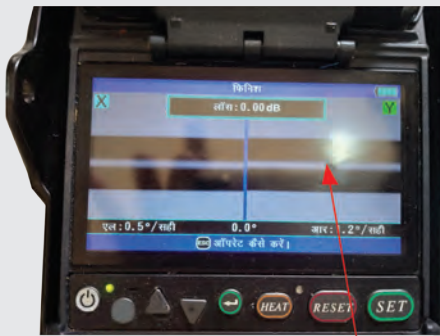
Fig. 5.34(a): Pressing the set button
