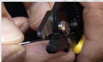
Fig. 4.19: Hold the fibre with the help of stripping tool
