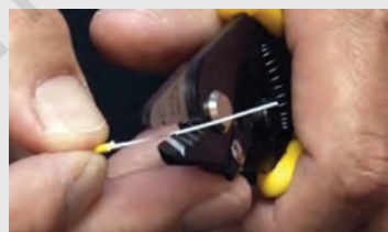
Fig. 4.20: Removal of the jacket of the optical fibre
