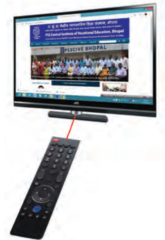
Fig. 2.14: Infrared light is used in TV remote
