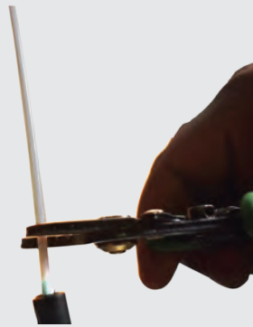
Fig. 5.13: Stripping tool removing the fibre tube
