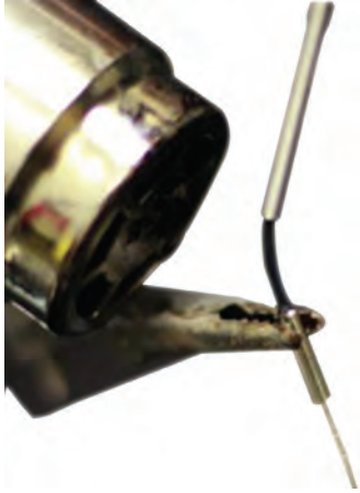
Fig. 4.27: Ferrule inserting into the optical fibre cable
