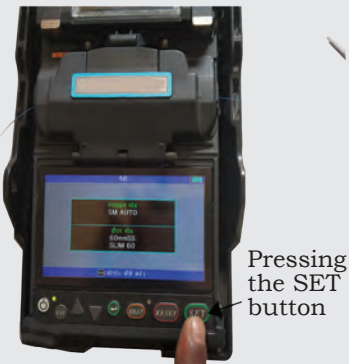
Fig. 5.34(a): Pressing the set button
