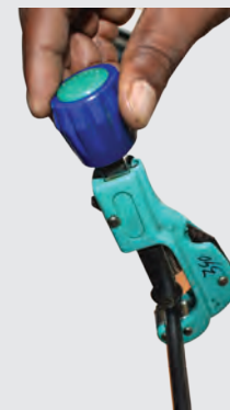
Fig. 5.10: Working of round cutter on the fibre
