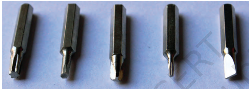
Fig. 4.3: Interchangeable tips of screwdrivers
