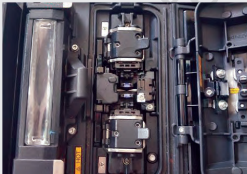
Fig. 5.30: Fixing the fibre inside the machine by closing the left clamp
