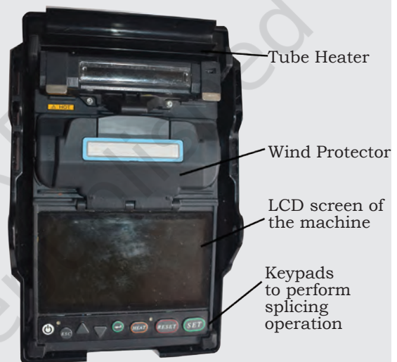
Fig. 5.24: Components and parts of the splicing machine
