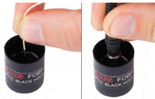
Fig. 4.30: Matching gel using for index matching
