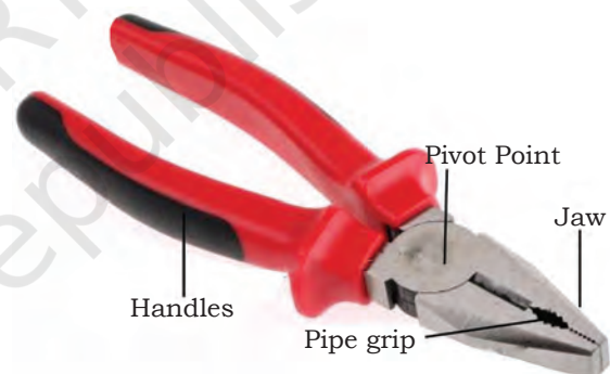
Fig. 4.10 Combination plier and its parts
