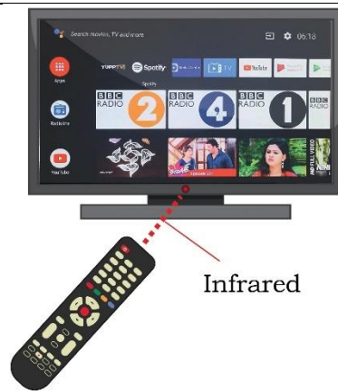
Fig. 3.5: Infrared light wave used in television remote
