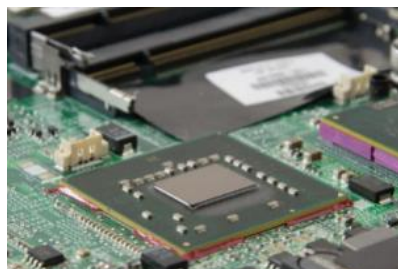
Fig. 1.9: A GPU on a PCB board
