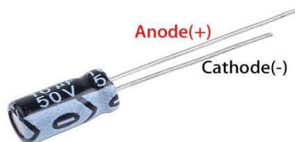
Fig. 3.7: Polarity of electrolytic capacitor
