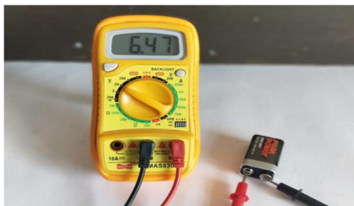
Fig. 4.13: Measurements of DC Voltage
