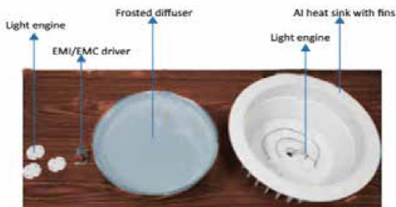
Fig. 2.23: Down Light Assembly parts
