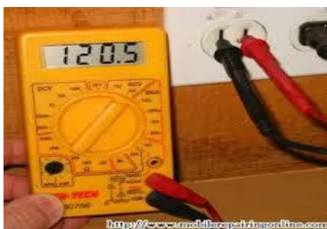
Fig. 4.12: Measurements of AC Voltage
