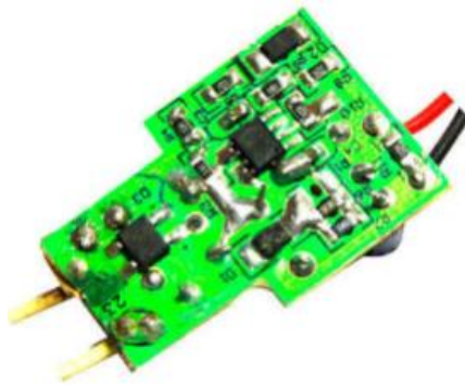
Fig. 2.11: LED driver in Housing
