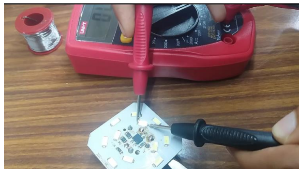
Fig. 2.9: Check all the LEDs
