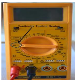
Fig. 4.16: Continuity Test using Multimeter
