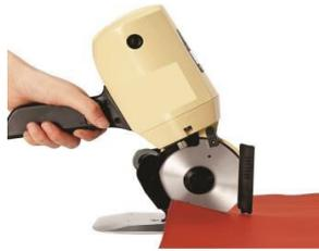
**Fig 1.32 Round Knife cutting machine**
