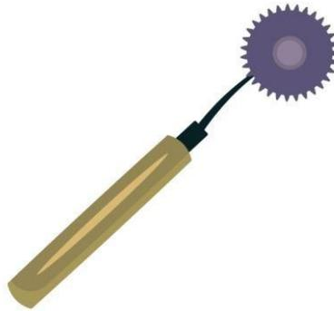
**Fig 1.10 Tracing Wheel**
