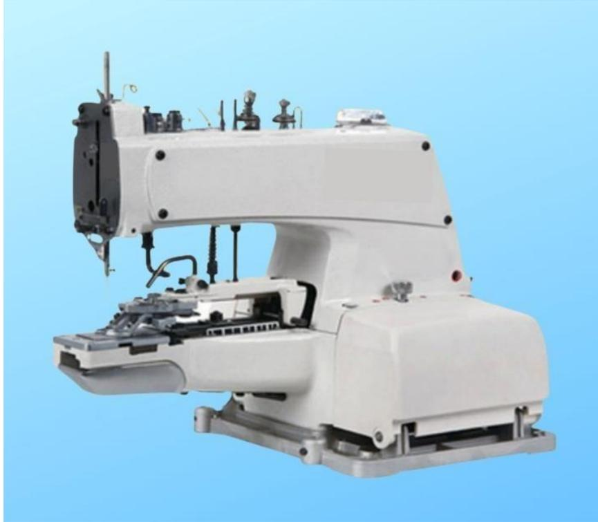
**Fig 1.52 Button Attaching machine**
