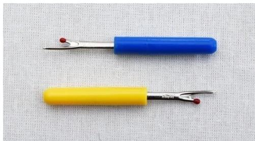
**Fig 1.22 Seam Ripper**
