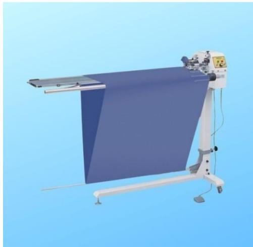
Fig 1.37 Rib cutting machine
