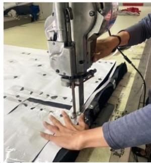
Fig 1.30 Straight Knife cutting machine
