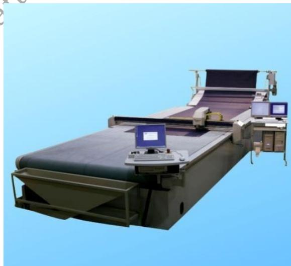
**Fig 1.36 Computer controlled knife cutting machine**
