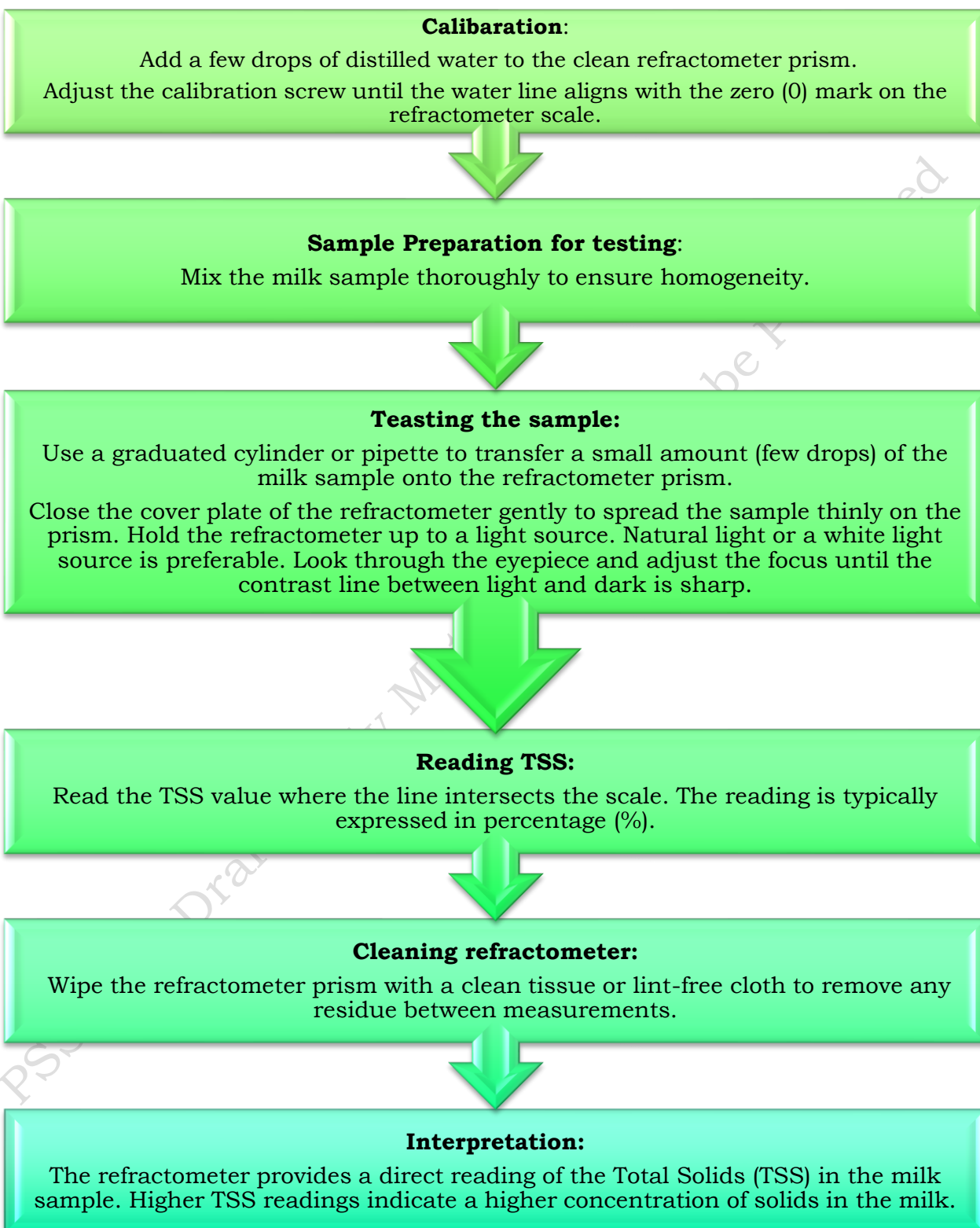
Fig. 5.5: Total Solids (TSS) Analysis Using a Refractometer
