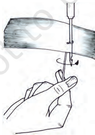
Fig. 3.1(f) Chain stitch formation (step-6)
