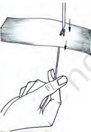
Fig. 3.1(e) Chain stitch formation (step-5)
