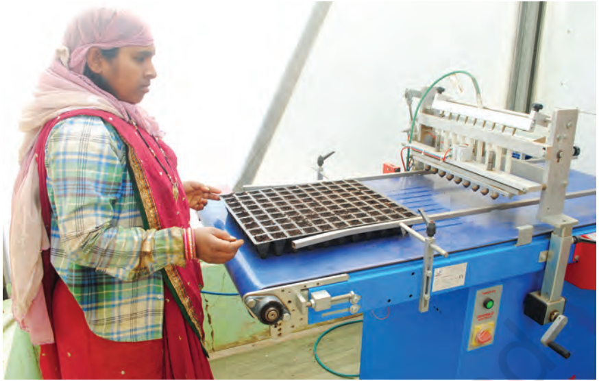
Fig. 2.8: Seed sowing by machine in plug-trays
