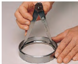
Checking inside groove
