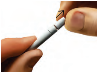
Fig. 9.11 Pull the outer shield of the cable
