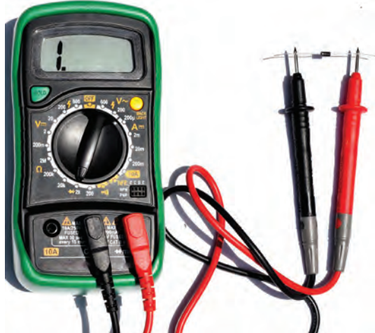
Fig. 2.32 Diode in reverse bias condition
