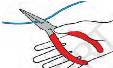
Fig. 9.24 Hold the wire using a pair of pliers
