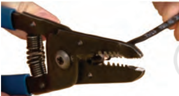
Fig. 9.61 Strip off the insulation
