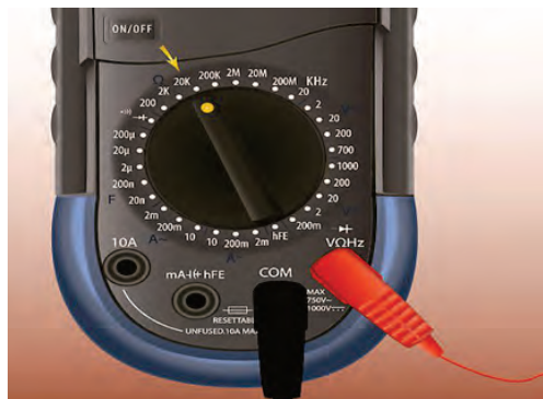
Fig. 7.2 Twisting the selector knob
