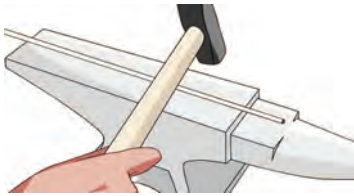
Fig. 9.42 Straightening the wire using a hammer
