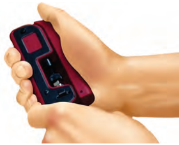
Fig. 9.16 Crimp the connector using a cable crimper
