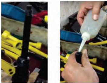
Fig. 9.60 Fill oil in the hydraulic crimping tool
