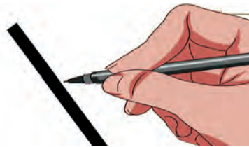
Fig. 9.29 Marking on the wire for bending
