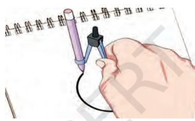
Fig. 9.38 Curve template drawn using a compass
