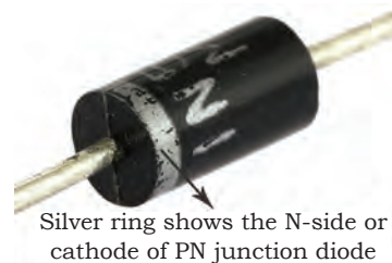
Fig. 2.24 Silver ring in diode
