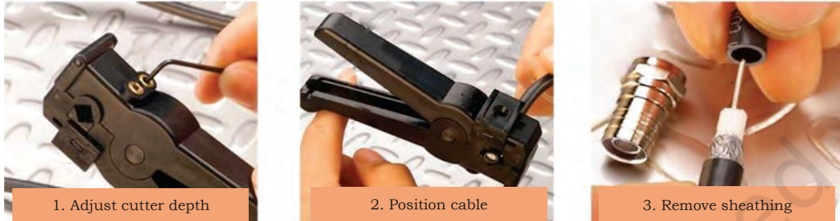
Fig. 9.74 Insulation stripping of a coaxial cable
