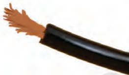
Fig. 9.62 Twist the conductor
