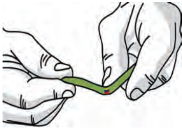
Fig. 9.28 Put a cut mark around the wire and bend it up and down to break
