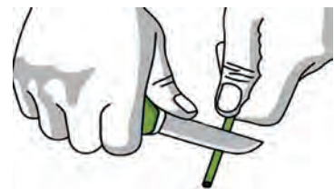
Fig. 9.26 Place a utility knife on the wire that needs to be cut
