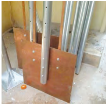
Fig. 4.8 Copper plate used for plate earthing
