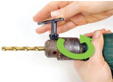
Fig. 7.21 Turn the chuck key counter clockwise
