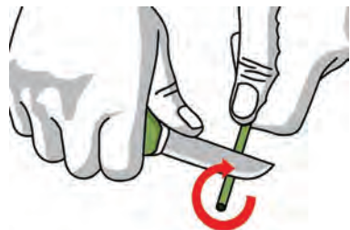
Fig. 9.27 Roll the wire with one hand
