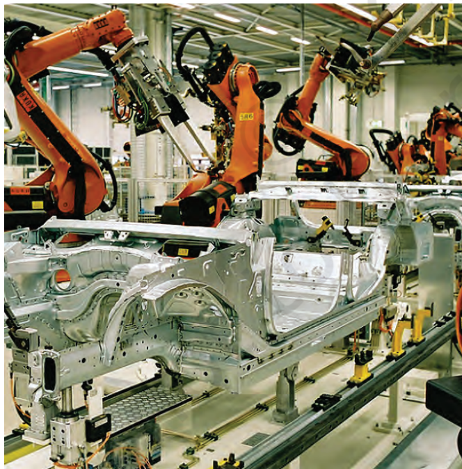
Fig. 8.1 Assembly line in the automobile industry uses electromechanical assembly
