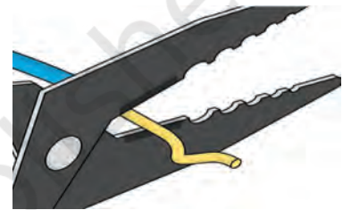
Fig. 9.25 Cut the damaged part of the wire
