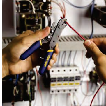
Fig. 9.4(b) Stripping a wire using a non-adjustable stripper
