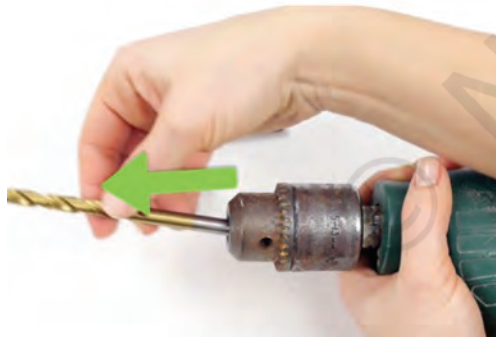
Fig. 7.22 Slide the drill bit out
