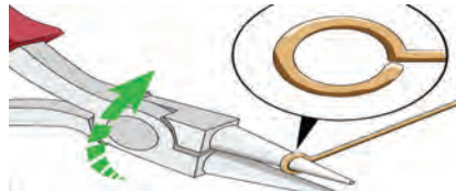
Fig. 9.49 Bending the nose of wire using a nose plier
