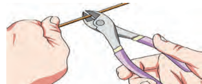
Fig. 9.50 Cutting the extra wire with a wire cutter
