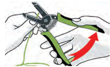
Fig. 9.21 Press the handles of the stripper to remove insulation
