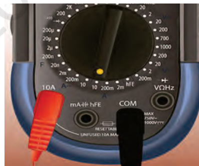
Fig. 7.9 Probes of multimeter connected to current measurement slot
