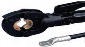
Fig. 9.72 Crimped cable with crimper
