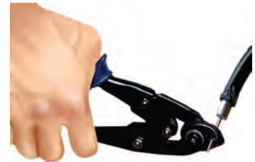
Fig. 9.14 Cut the wire using a wire cutter
