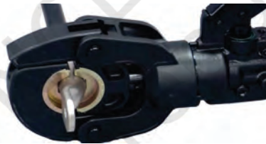
Fig. 9.70 Inserting the cable into the crimper
