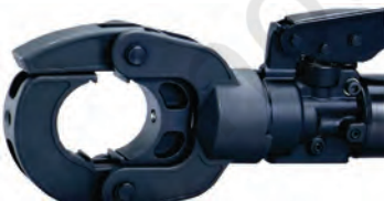
Fig. 9.73 Dies removed from crimper
