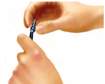
Fig. 9.15 Insert a connector in the cable conductor
