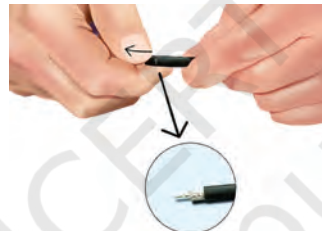
Fig. 9.12 Pull the inner cut of the cable
