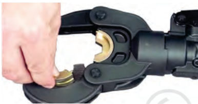
Fig. 9.69 Fixing the dies in crimper
