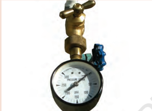
Fig. 4.41: Pressure release valve
