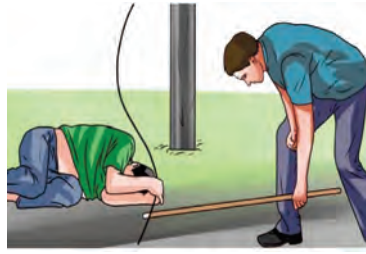
Fig. 6.6: Insulating material must be used while rescuing the victim
