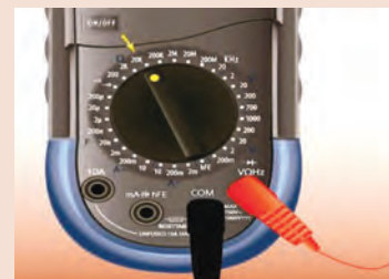
Fig. 3.3: Measuring the resistance of resistor by touching the resistor terminal to the red and black probes
