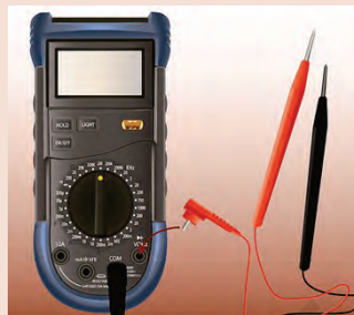
Fig. 3.5: Connecting the red probe to the volt terminal and black probe to the common terminal
