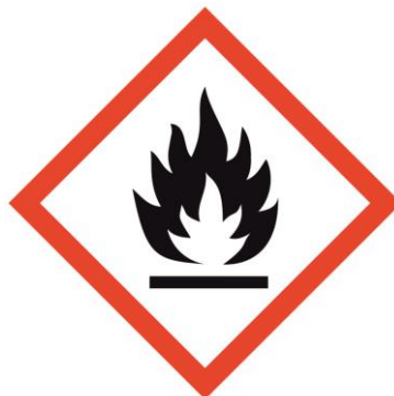
Fig.: 5.17 - Flammable substance Sign
