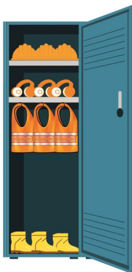
Fig.: 5.8 – Proper Storage Facility for PPEs
