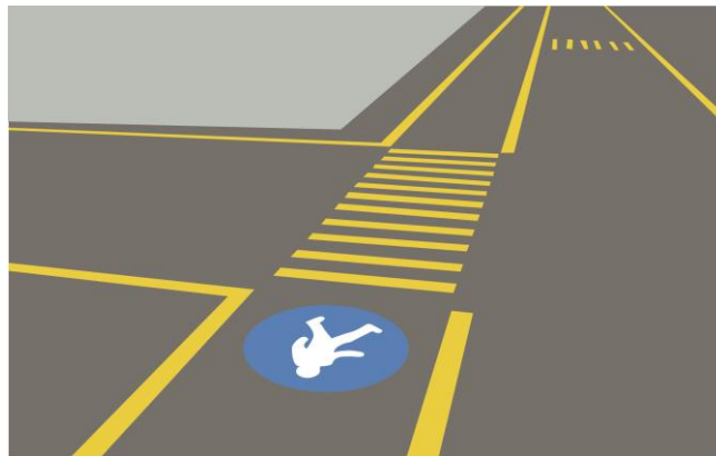
Fig.: 5.3 – Yellow Demarcation for Pedestrian Pathway
