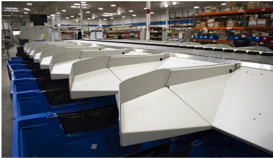
Fig. 2.15: Chutes and slides used for sorting
