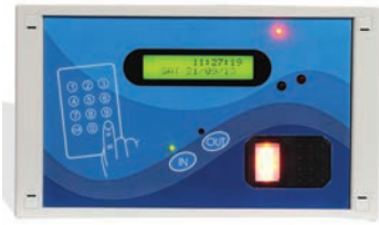
Fig. 2.51: Wall mounted biometric LAN based fingerprint device
