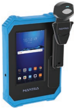
Fig. 2.23: Integrated iris scanner
