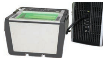
Fig. 2.29: Fingerprint scanner connected and ready to capture biometric data
