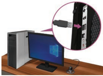
Fig. 2.30: Connecting web camera to computer system through USB connector
