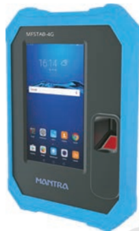
Fig. 2.22: Integrated fingerprint biometric machine
