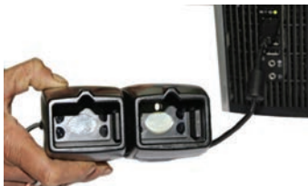
Fig. 2.33: Iris scanner connected to the computer and is ready to capture iris
