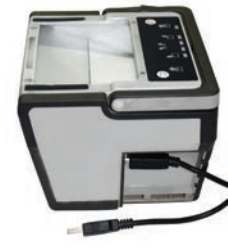
Fig. 2.27: Data cable of scanner device
