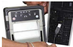
Fig. 2.28: Connecting fingerprint scanner to computer through USB connector
