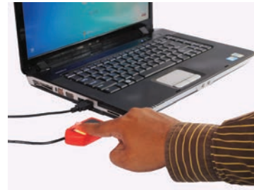
Fig. 2.58: Fingerprint scanner connected to the computer
