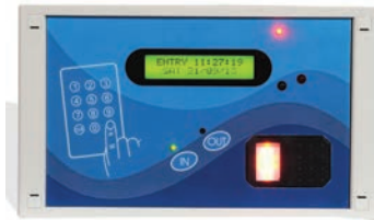
Fig. 2.21: Biometric LAN based fingerprint device
