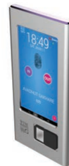
Fig. 2.19: Android based biometric attendance system
