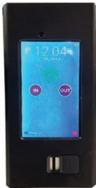
Fig. 2.52: Wall mounted android based fingerprint device
