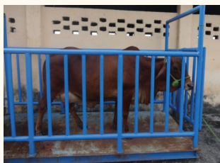
(a) A platform type electronic weighbridge is used to measure the weight of an animal.
