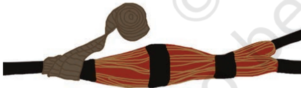
Fig. 5.10 Wrapping the cable with mesh tape
