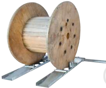
Fig 4.18 Cable drum without cable
