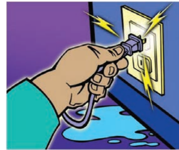
Fig.3.26 Avoid water while working with electricity
