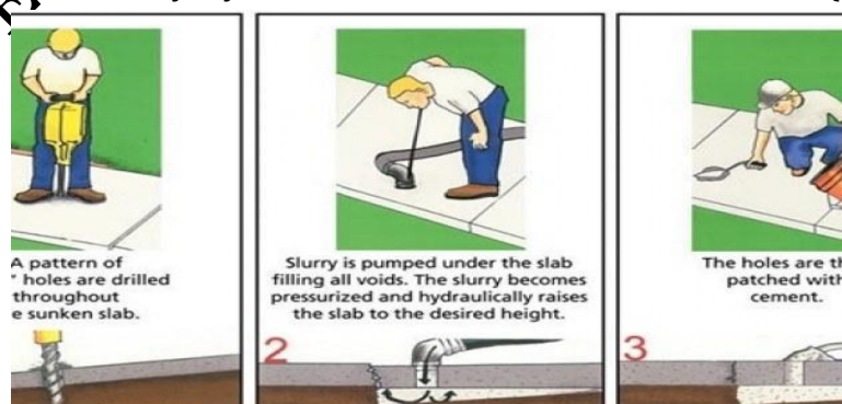
Fig.3.32: Process of Grouting
