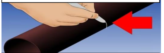
Fig.3.15: Marking of pipe by chalk
