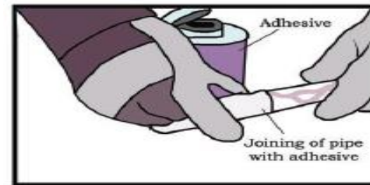
Fig.3.18: Joining of elbow after application of solvent
